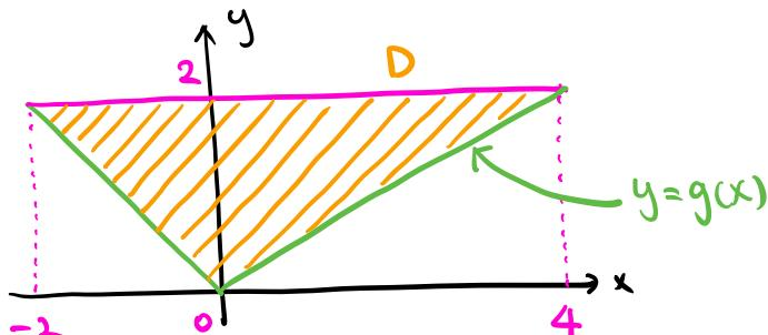
$$\Rightarrow \iint_D 2xy \, dA = \int_{-2}^4 \int_{g(x)}^2 2xy \, dy \, dx.$$
